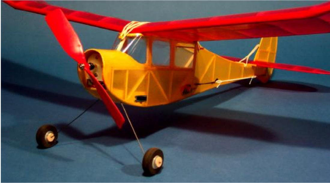
This is my Viking built for FAC Old Time Gas Replica (OTGR) competition. It is from the Al Lidberg kit. A Hiline Mini-6 and a battery of 3 cells of 110 mAh capacity powers the plane. The model has 108 square inches of wing area and, with the power system described, weighs 77.6 grams.
