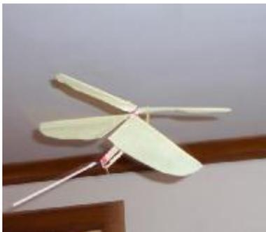
This little flapping-wing model is called the Mayfly. When I started building it, I figured it may fly, or it may not! After trying a variety of different wing designs, finally it does fly, and quite well in fact. The biggest challenge was coming up with a design for the front wing since there is so little root chord to support the tissue.
