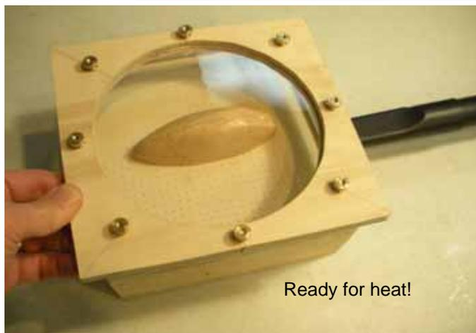
I modified Chris's design slightly by using 1/2" rather than "1x" (actually 3/4") pine which I found at the local Lowes store. The only tedious part was drilling the many 1/32" holes in the top piece. To do this, I stuck a piece of 1/4" grid graph paper to the 1/4" plywood with a removable glue stick, and drilled away with a Dremel drill press. Doing this a little at a time, rather than all at once, made the job less daunting.
