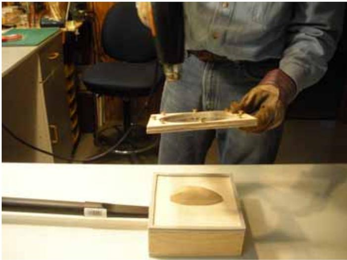
I used a variable temperature heat gun to heat the plastic. Test first on a scrap piece to determine the temperature setting at which the plastic will sag but not melt through. I found it best to as much as possible get the entire sheet heated uniformly so the vacuum force applies to the piece evenly. Note the leather glove. A stove top burner, if convenient, may be another good way to heat the plastic uniformly, but I have not tried this.
