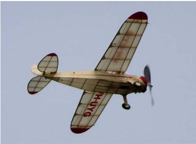
Lo and behold the model now exhibits a much more consistent behavior with its enlarged tail feathers. Climb out had typically been pretty good. Now the model glides much more consistently except when the motor bunches in the rear. An adjustment to the motor stop has already helped with that. Although the Cessna will not likely turn in consistent max flights, it should be able to produce 90 seconds consistently. Here's hoping anyway.
