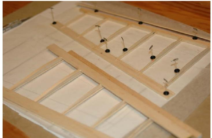
Color photo shows the new wing under construction. Leading edge is made from relatively hard balsa. Remaining components are all of light weight 1/16" stock. Sheeting on top leading edge and trailing edge made of two pieces of sheet balsa (on top and bottom of rib) should make for a very stiff wing. Bottom and top cap strips help as well. All up weight should be low even though it is a bit thicker than a quarter inch before sanding.
