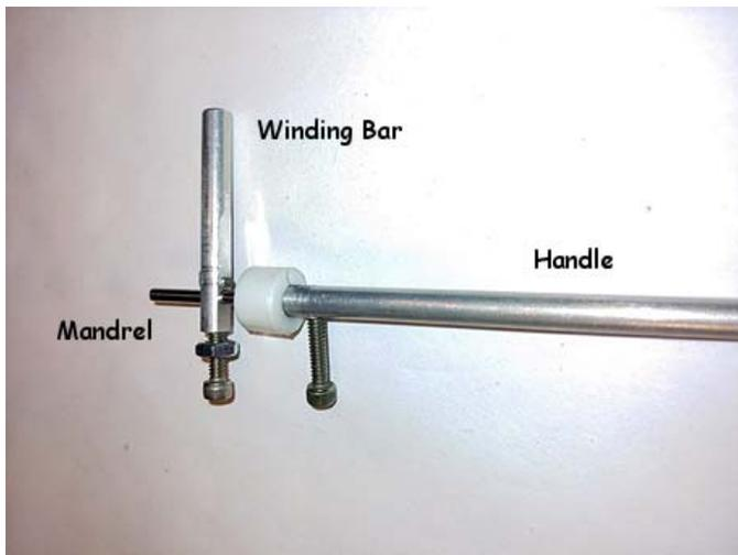
The Handle is a length of 1/8" thick wall aluminum tubing. The white nylon bushing ring was added to provide a larger face surface against which to wind the spring. A piece of drill rod serves as the Mandrel. The thick wall of the Handle was drilled and tapped to accept a set screw to hold the Mandrel in place.
