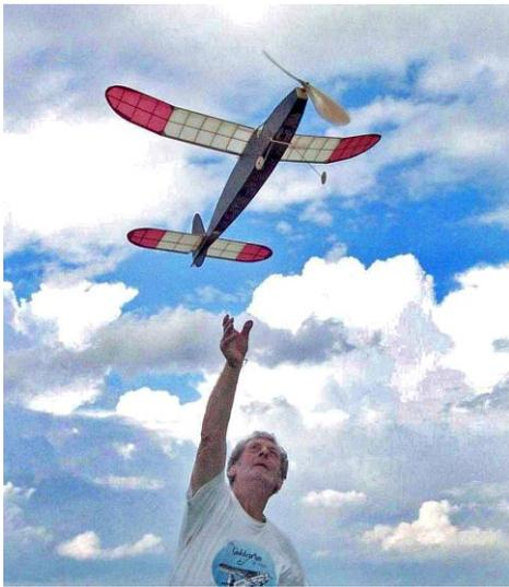
Above: An outdoor endurance model is launched. The model has a wingspan of 36 Inches and uses multiple loops of rubber strip for power. Below: This is the *Squirrel*, a beginner's model that's easy and quick to build and is a fine flier. See page 5 for more information on the *Squirrel*.
