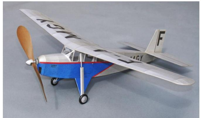
Here's a 24" rubber-powered scale model of a 1932-era French lightplane. Below: An engine-powered contest model is launched showing its high-angle climb. A timer will shut off the single-cylinder motor after a pre-set number of seconds.
