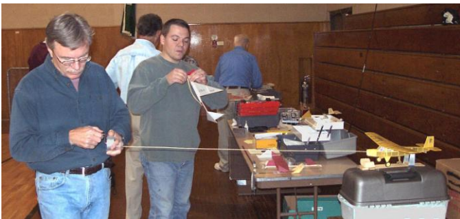
The rubber motor of this small scale model is stretched to permit the maximum number of desired turns to be added. The model is anchored securely in a winding "stooze" (see glossary) mounted on the flier's field box. He'll slowly start coming in toward the model as he completes the second half of the desired turns. He'll then transfer the rubber motor to the propeller hook, detach the model from the stooze, and be ready to fly. For long flights, proper winding technique is important.
