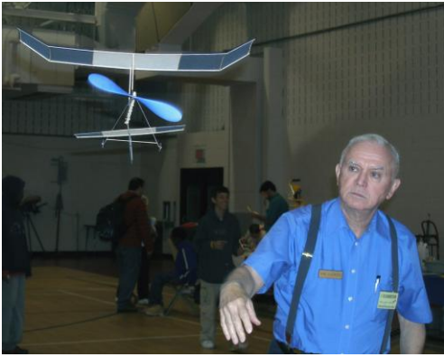
A basic indoor endurance model is seen just after being launched. It has a molded plastic propeller, a solid balsa stick for a fuselage, and tissue covered wings and tail framework.
