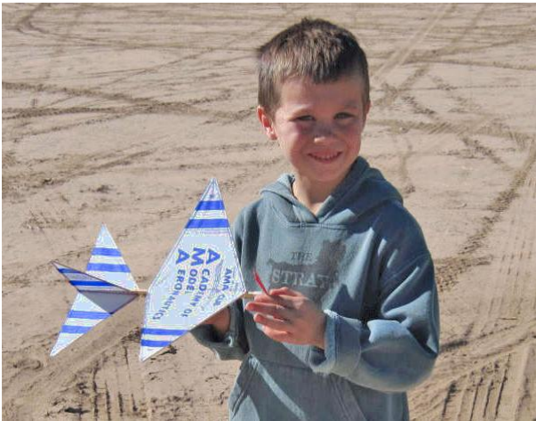
This is the AMA Cub. It's an easy-to-build beginner model. See the vendor list for more information. The balsa wood framework is glued direct to the plan, which then becomes the model's covering after careful trimming around the outlines with a single-edge razor blade.
