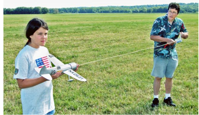
Rubber powered models are wound using a mechanical winder and by stretching the rubber motor to enable more turns to be put in for a long motor run. 1,000+ turns are not uncommon!
