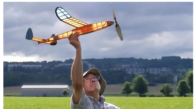
A flier launches his non-scale rubber-powered endurance model. The wound rubber motor can be seen through the translucent tissue covering. The SUNY Geneseo campus is in the background. The large diameter propeller is typical of these models.
