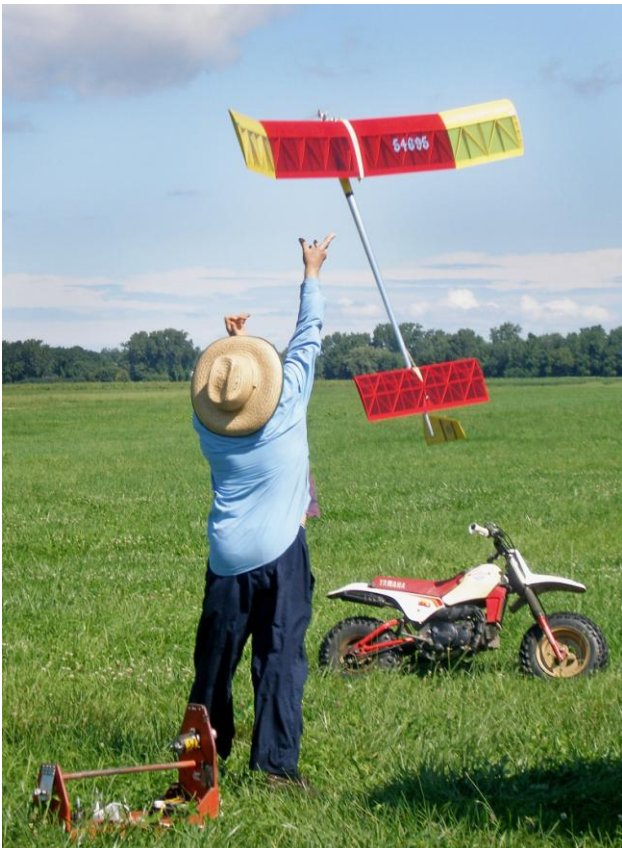
This model uses a single-cylinder reciprocating engine as its power plant. The flier's toolbox rests in the grass while his small motorcycle waits to take him downwind in pursuit of the model. Lots of thrust from the motor allows a fast vertical climb. An onboard timer shuts it off.
