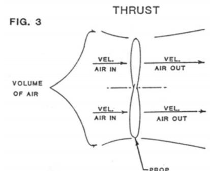
$$\text{THRUST} = \text{VELOCITY OF AIR OUT} \\ \text{MINUS VELOCITY OF AIR IN} \\ \text{TIMES THE VOLUME OF AIR MOVED}$$
