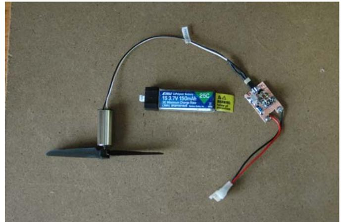
Motor, propeller and motor run timer as provided by Willamette Modelers along with 150 mAh LIPO battery from Horizon Hobby. These are the components used for the measurements described in this article. Note, this is a sample of one and a sample of one is next to none.
