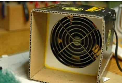
To keep the filter material from getting too close to the fan, a cardboard panel was cut from a scrap of photographich matt board. Any thin cardboard or corrugated should work. Cutting a round hole was a bit tricky but a perfect circle is not really needed. Corrugated stops are located on the fan side of the panel to keep the fan from sliding against the panel. A stop is all the more important if your fan does not have a grill as shown here.
