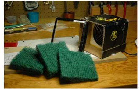
Fabricating the enclosure is easily done using corrugated cardboard from most any source. Cardboard from a shoe box was used for the collector pictured. One of the dimensions of the shoebox matched the fan size exactly. Folds had to be made for the other edges of the fan to form an enclosure about 6 inches long by 5 inches square. Woodworker’s yellow glue was used for gluing up the cardboard.
