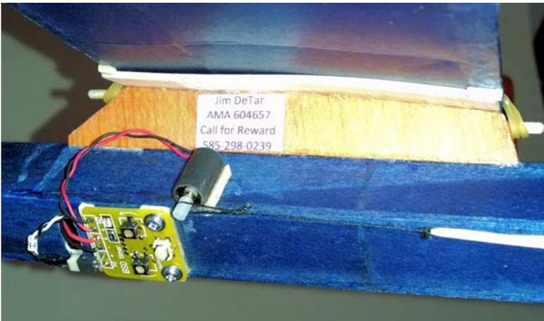
Closeup showing Jim's installation of the Bob Selman motor run timer and DT mechanism. This is an alternate to the Willamette Modeler's system.
